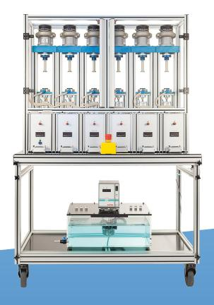
Test equipment to masticate chewing gums, especially medicated ones, for the in vitro release of substances from the samples into a surrounding liquid medium. Up and down strokes (vertical) of the lower jaw in combination with a revolving movement of the upper jaw which provides mastication of the chewing gum and at the same time an agitation of the test medium.
