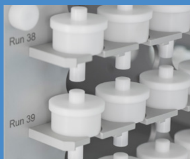
10 or 40 Batch sample magazine for continuous testing 24/7.
