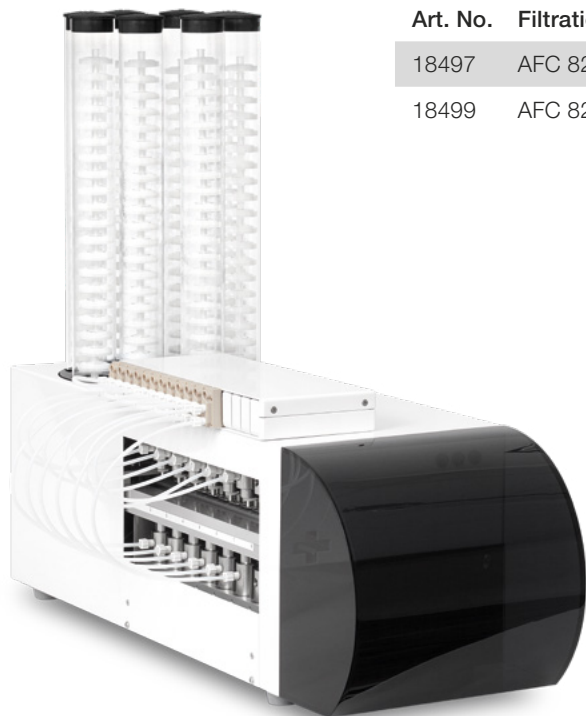
AFC automatic membrane filter exchange system
